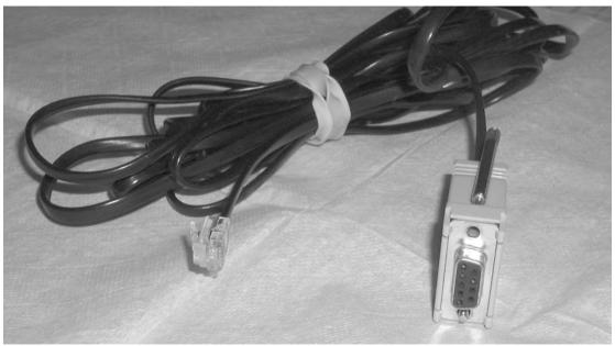
Plug the telephone plug (RJ11) end into the RS232 PORT jack on the Time Machine and the 9 pin computer plug (DB9) into your computer's communications port, normally called COM1 or COM2.
